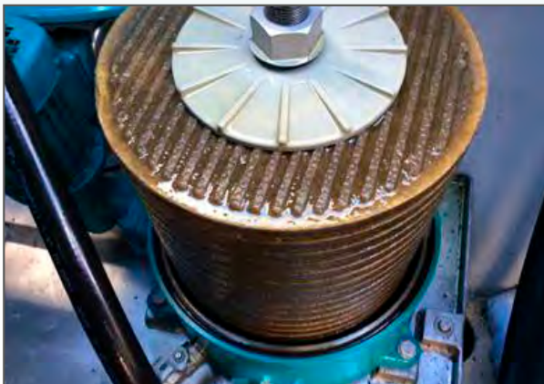
Even a large oil filter is drained within minutes. Installation at E.ON Wind Services
