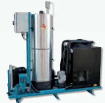
Varnish Removal Unit
